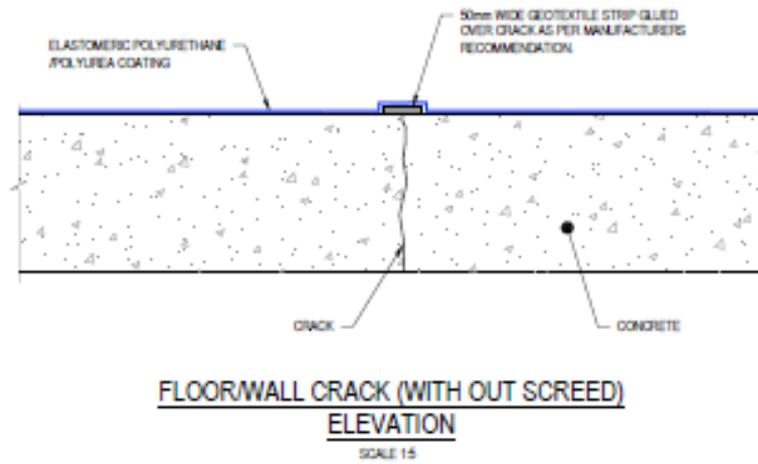
**Figure 6: Groove Detail at Floor or Wall Crack**
