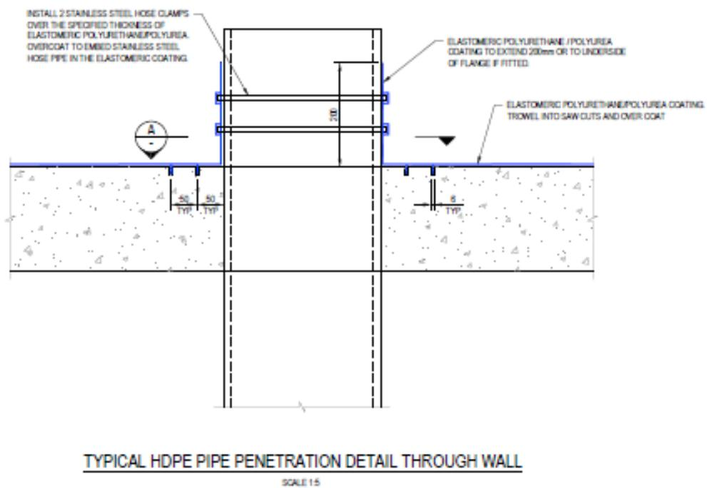
**Figure 7: Groove Detail at Typical Pipe Through Penetration**
