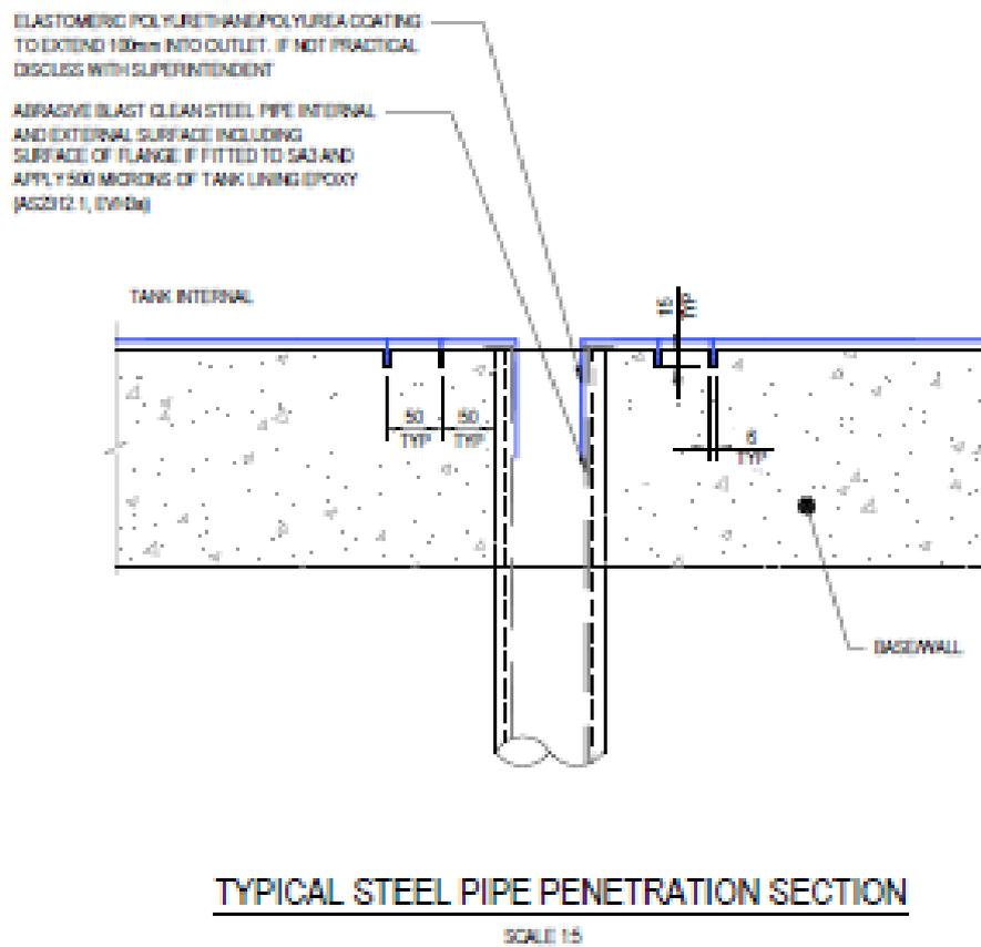
Figure 9: Groove Detail at Flush Pipe Penetration
