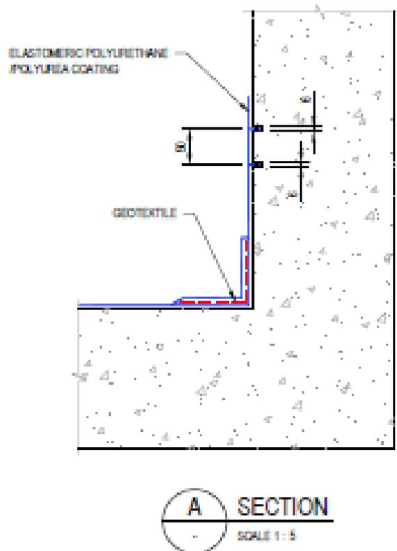
**Figure 5: Groove Detail at Wall to Floor Intersection**
