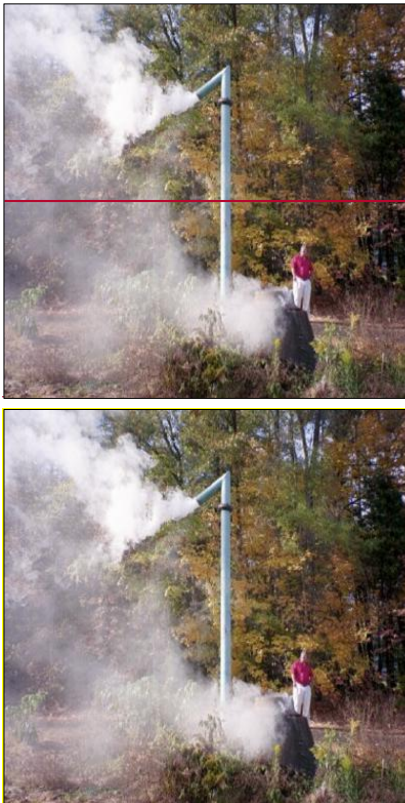
Figure 12: Uncontrolled air release caused by hydraulic surge
