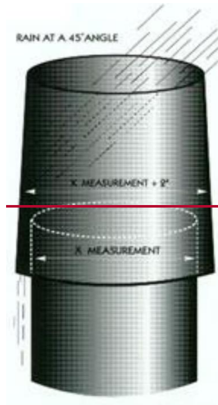
Figure 12-1 Collar-type rain guard for a stack
