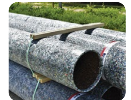
PVC pipe manufactured using material from recycled PVC.
