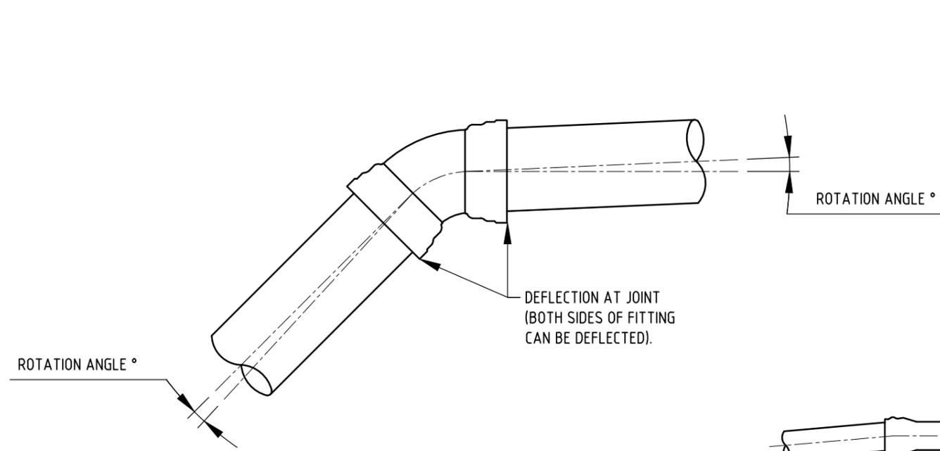
TYPICAL DEFLECTION AT PIPE TO FITTING JOINTS
