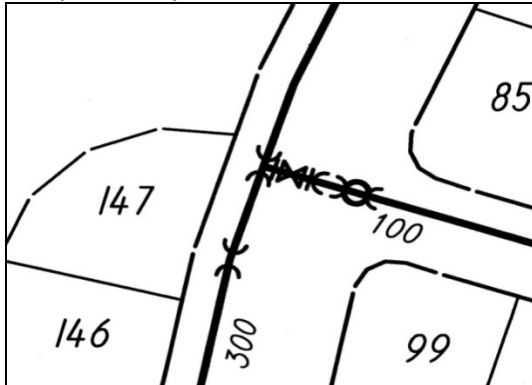
Sample 1: Stop valve in branch water main
