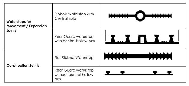
Figure 1 Various types and shapes of waterstops
